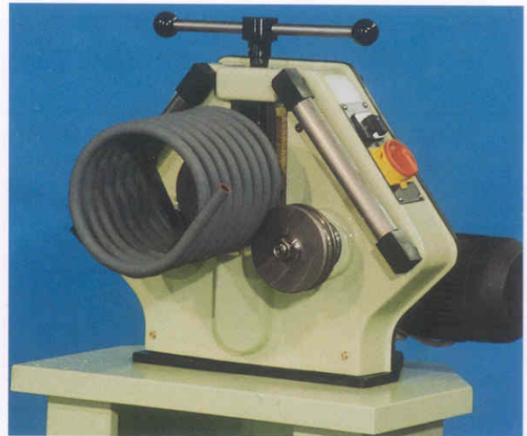
Small tubes may be rolled for use in heat exchangers or cooling systems, as well as many other applications.
