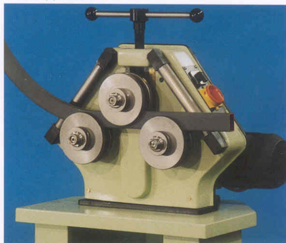
Square or rectangular tubes, larger than 1 1/4", require optional roll discs for added support to tube walls.
