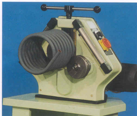
Small tubes may be rolled for use in heat exchangers or cooling systems, as well as many other applications.
